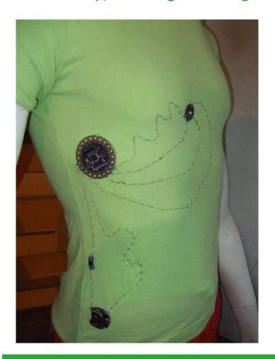
Use conductive thread, LEDs, batteries and programmable electronics to make your own creation
